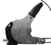
Figure 3: Tensioning the belt
