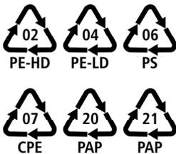
The printed or embossed markings indicate the materials which were used: PE stands for polyethylene (code 02 means high-density PE, 04 stands for low-density PE), PS stands for polystyrene and CPE for chlorinated polyethylene. PAP 20 means corrugated cardboard and PAP 21 other cardboard. All plastics are thermoplastics which are very easy and efficient to produce. They are also very easy to recycle and therefore can even have a smaller ecological footprint than comparable cardboard packaging.
