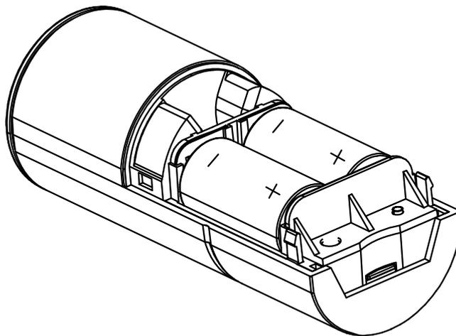
Once the batteries have been inserted, the device will start flashing for initialisation. Meanwhile, the signal lamp (**C**) lights up red several times and the acoustic signal for “disarmed” is triggered. Afterwards, the device is ready for operation.
