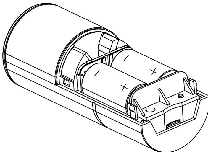
Once the batteries have been inserted, the device will start flashing for initialisation. Meanwhile, the signal lamp **(C)** lights up red several times and the acoustic signal for “disarmed” is triggered. Afterwards, the device is ready for operation. You can immediately operate the siren via the teach-in button **(E)**.
