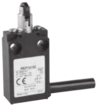
Rollenstößel quer MEP1G14* G14: Metallrolle G15: Nylonrolle
